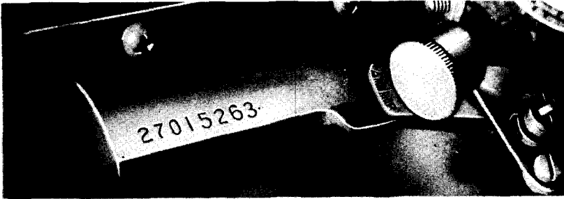
ENGINE SERIAL NUMBER—ON RIGHT SIDE OF BLOCK
