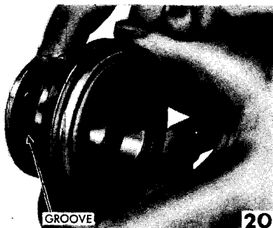
RELEASE BEARING FORK GROOVE—WB Apply light coat of grease to fork groove in release bearing support. Do not fill groove.
