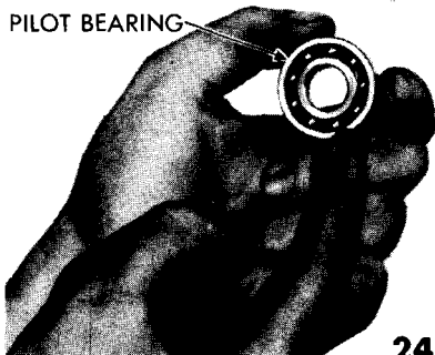
CLUTCH PILOT BEARING—WB Hand pack bearing with grease, being sure that all balls and races are coated.
